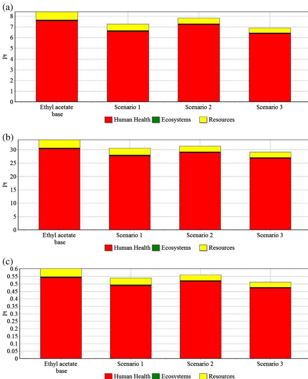
Fig. 5. Severity of damage categories for the recovery of (a) hydroxytyrosol, (b) tyrosol, and (c) TPb from OMW using ethyl acetate as the solvent. Proposed scenarios: (1) addition of 8% Na<sub>2</sub>SO<sub>4</sub>; (2) production of ethyl acetate from bioethanol; (3) combination of scenarios 1 and 2.
