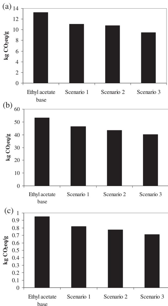
Fig. 6. Global warming potential (GWP) in CO<sub>2</sub> equivalents for a timeframe of 100 years for the extraction of 1 g of (a) hydroxytyrosol, (b) tyrosol, and (c) TPB from real OMW using ethyl acetate as the solvent. Proposed scenarios: (1) addition of 8% Na<sub>2</sub>SO<sub>4</sub>; (2) production of ethyl acetate from bioethanol; (3) combination of scenarios 1 and 2.
